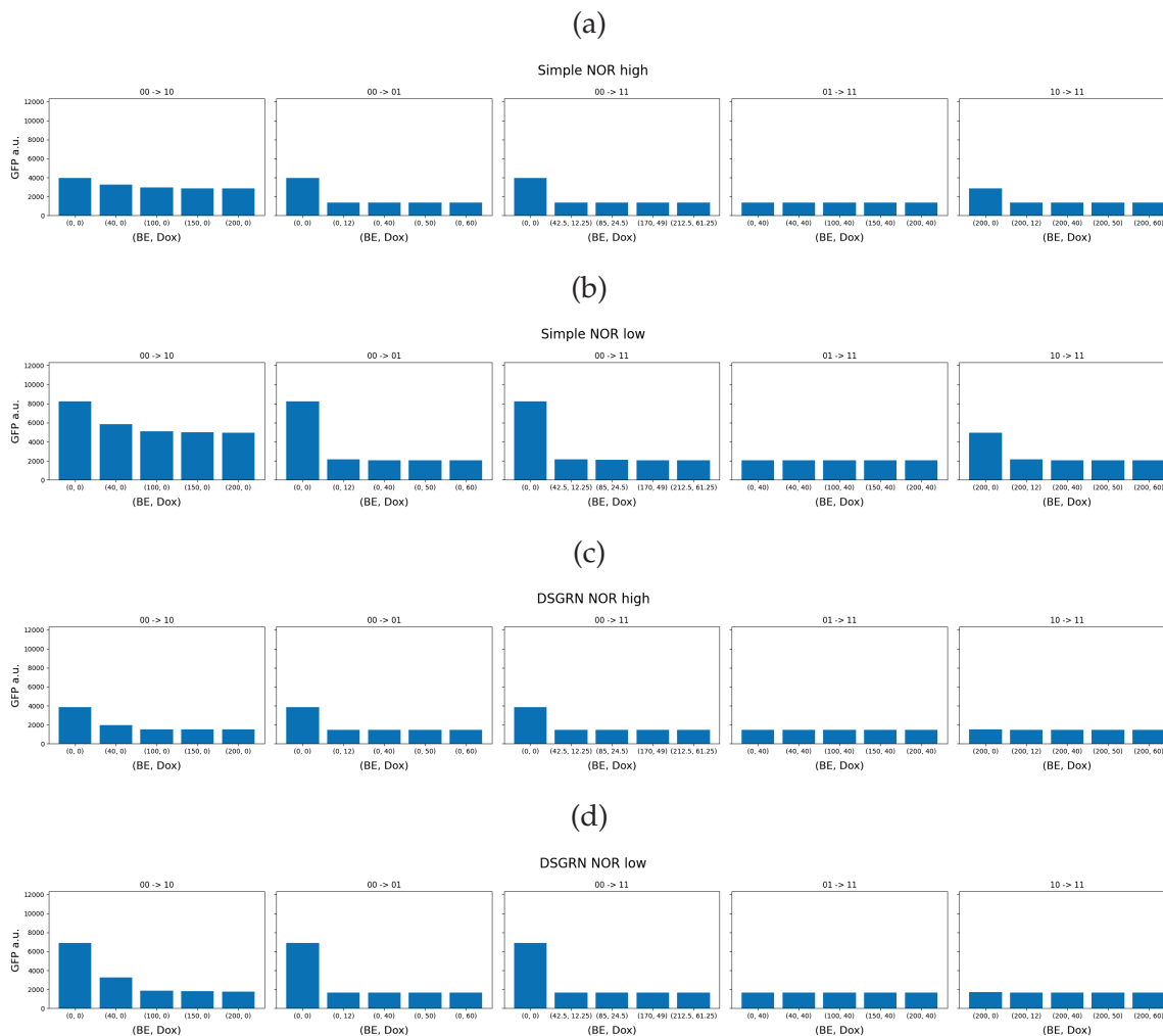
Figure 6.7. Predicted steady-state values of the geometric mean of the flow cytometry distribution of GFP a.u. using estimated Hill function parameter values for: (a) Simple NOR/CDM low design, (b) Simple NOR/CDM low design, (c) DSGRN NOR/CDM high design, and (d) DSGRN NOR/CDM low design. An OFF circuit state corresponds to approximately 1500-2000 a.u.; robust ON circuit states occur at about 8000 a.u. and up, and weak ON states occur at about 4000 a.u. Columns 1-3 (transitions 00 \rightarrow 10 , 00 \rightarrow 01 , 00 \rightarrow 11 ): The left-most bar in each bar graph should be ON. All other bars should be OFF. Columns 4-5 (transitions 01 \rightarrow 11 , 10 \rightarrow 11 ): All bars should be OFF.
